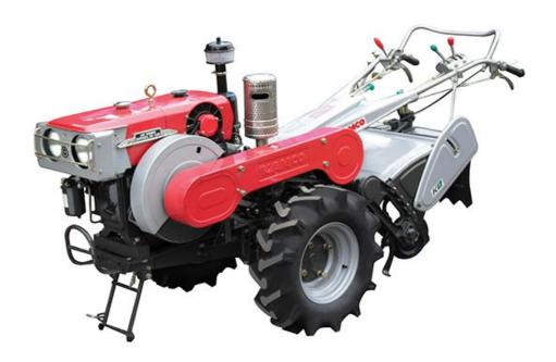
This compact engine is designed to generate continously 12hp of Powefor the most demanding jobs, and with a lower weight - per output Rating. The engine is perfected for low smoke level to satisfy Emission Norms conforming to even TREM-III norms. Reduced fuel consumption Per horse power output.
